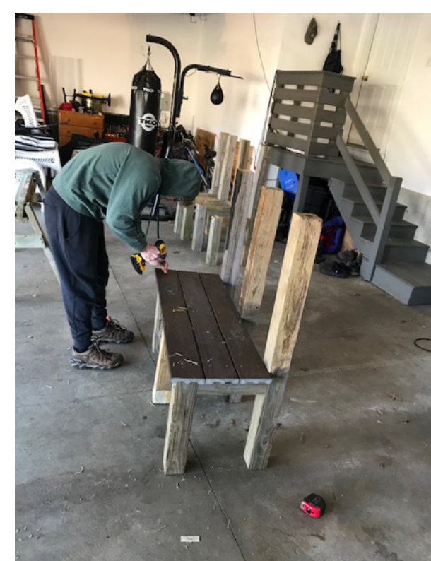
Anthony in his garage workspace, installing Trex seating to the benches. Anthony used posts from the old fence to create a solid bench frame.
